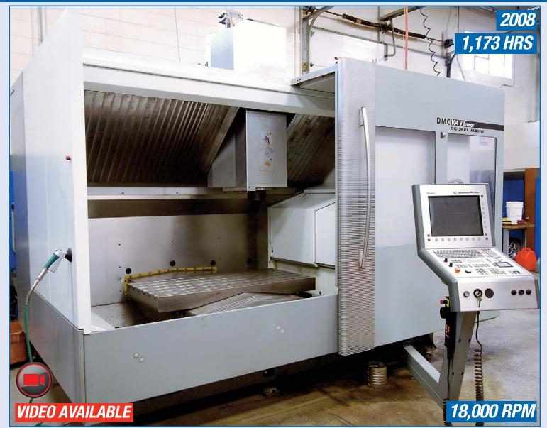
2008 **DECKEL MAHO** DMC 104V Linear CNC Vertical Machining Center, s/n 29110004964, DMG 3D Heidenhain i TNC530 CNC Control, 23-3/4" x 49-1/4" Table, Travels: X-40.94" (1040mm), Y-23.62" (600mm), Z-19.69" (500mm), A-3600, HSK-A63/SK40 Spindle, Speeds to 18,000 RPM, (30) ATC, Visiport VP220.C.FDX Brushless DC Spin Window System, Auger Chip Recovery, Chip Conveyor, Coolant Through Spindle, BMF Coolant System, 6,148 Power On Hours, 1,173 Run Time Hours
